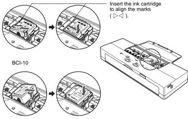
**7.** Press down gently on the high side of the ink cartridge until the ink cartridge clicks into the print head unit.
